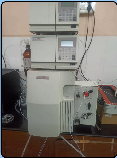
HPLC System with UV-VIS and RI Detector and Fraction Collector
